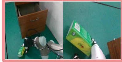
Figure 14: Special failure trajectory labeled due to robot–table collision.
